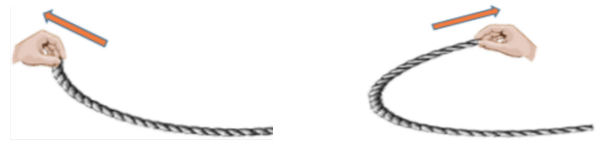
Fig. 1: An illustrative example of directional rigidity. Left: The rope moves almost rigidly when dragging it by one end to the left. Right: The rope deforms when pulling it on the right in the opposite direction.
