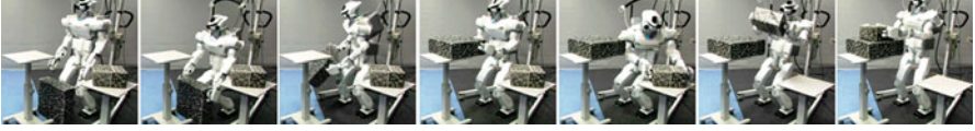
Fig. 11 Snapshots from the execution of the box stacking task on the HRP3 robot
